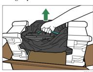
Holding the green handle, remove the protective materials from both ends, and then take the development unit out of the plastic bag.
