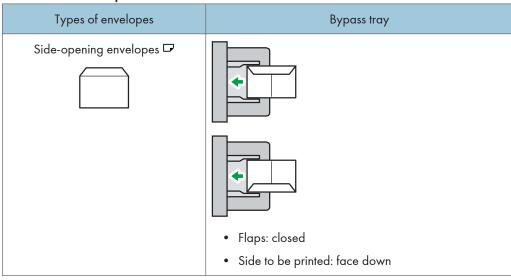
When loading envelopes, select "Envelope" as the paper types using both [Tray Paper Settings] and printer driver and specify the thickness of envelopes. For details, see "Printing on Envelopes", Print.
